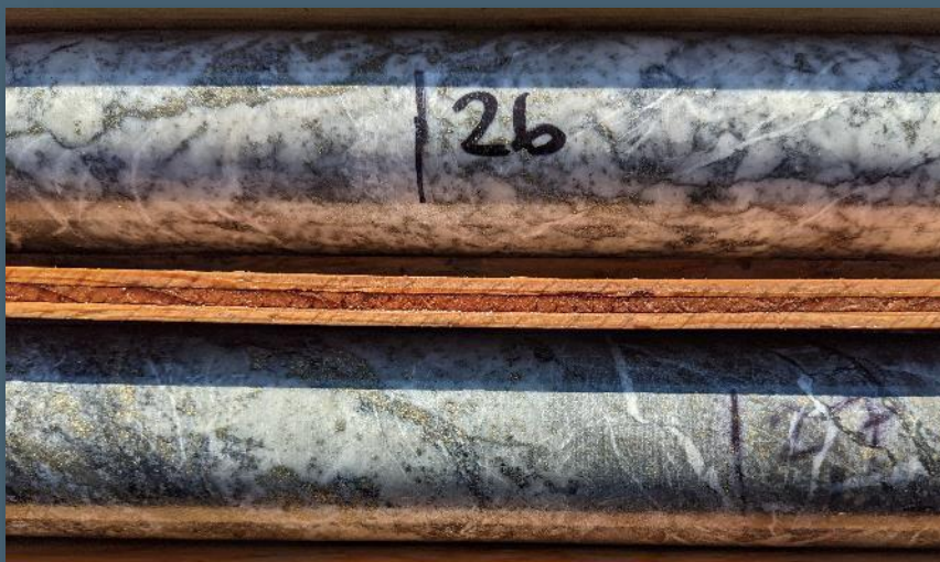
KH21-45 @ 26m: Gold-bearing Quartz-carb-sulphide veins
